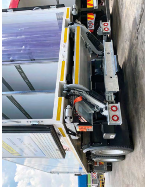
↕ DH-RM.20 heavy-duty fold-away lift • 1,500-2,000 kg Wide lift arm + 2 lift cylinders
