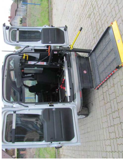
↑ DH-PH1.03 internal single arm lift • 300 kg
